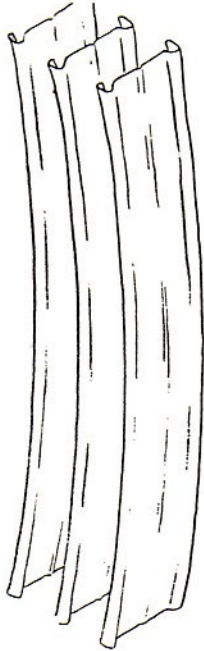
FIG. 4 "STRIP PLATE" DISTORTION
