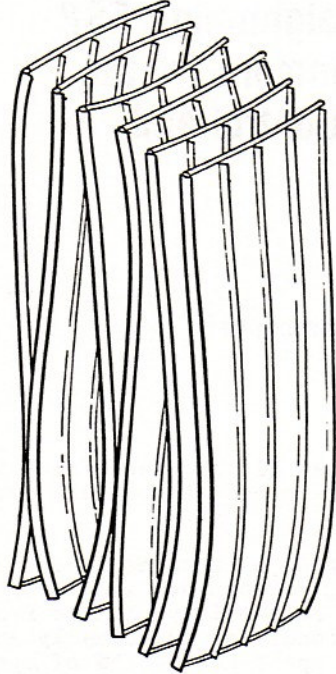
FIG. 1 COLLECTOR PLATE DISTORTION
